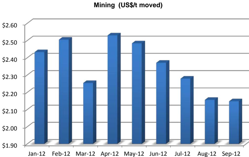
Improved drill and blast practices had a major positive impact on mining costs (see Figure 4), with the powder factor reduced by 20% over 2012 despite improved rock breakage and sizing being achieved.
